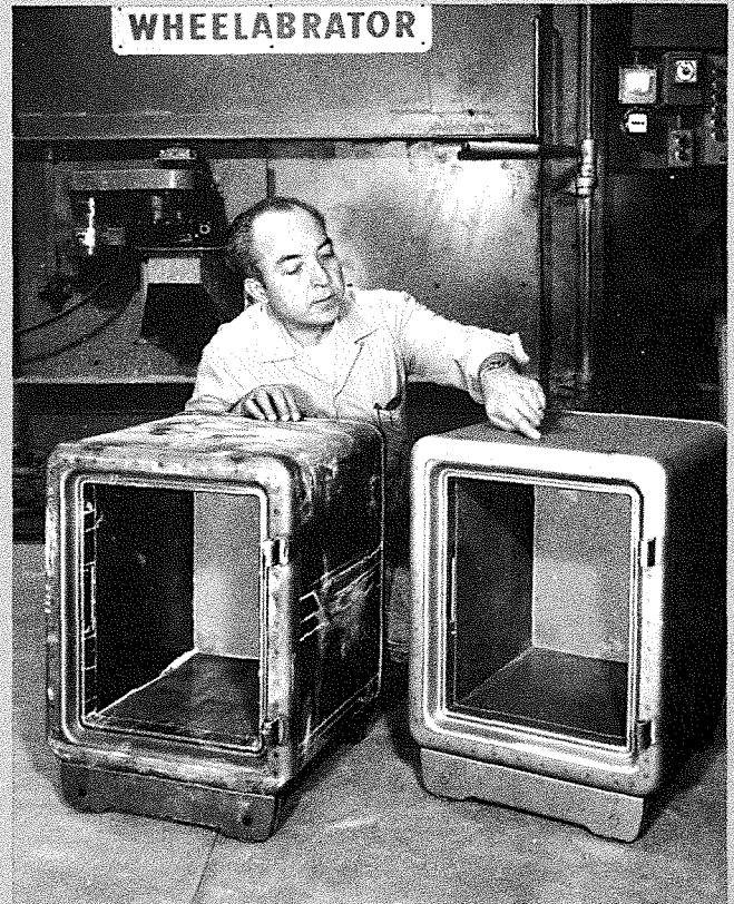
ABOVE — Safe before cleaning, left, and after a 30-sec. blast cleaning cycle in the Swing Table, right, dramatically illustrate the superb finish results obtained. The uniformly clean, matte surface provided by abrasive blast cleaning takes paint better, holds it longer and makes it more scratch-resistant. BELOW — 72" dia. Wheelabrator Swing Table, with four rotating auxiliary wheels, thoroughly blast cleans four 250-lb. steel safes or a variety of small components in a 30-sec. blast cycle.
